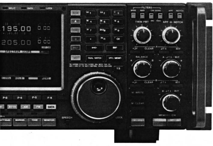
The IC-781 has a dual-watch function which allows simultaneous receive of two frequencies in the same band. Balance controls adjust VFO A/B receive strength levels. This feature is especially useful on Dx-expeditions or contests to check band activity or to tune in your next contact. The newly developed ICOM DDS (Direct Signal Synthesizer) system is incorporated to provide a fast transceiver lock-up time. This is essential for data communication systems.
