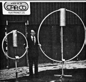
Tony Johnston G4OGP, pictured with two of his magnetic loop antennas, standing outside the Cap. Co Electronics factory at Skelmersdale
